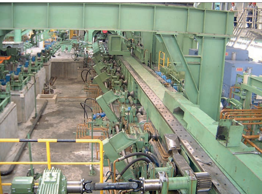
View of the entry side of a PQF® plant: inserter (front right in the picture) and retainer (rear centered in the picture)
