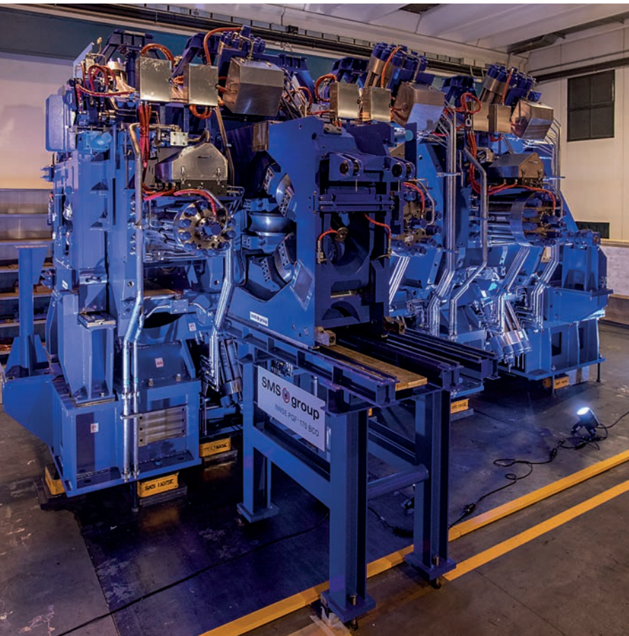
The 4 th generation 7-inch PQF® is able to roll 200 tubes per hour.
