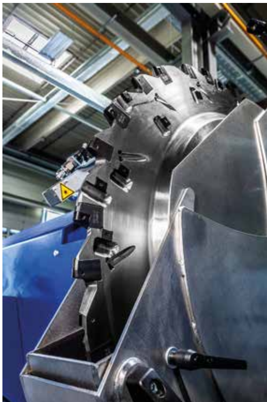
High-precision welding seams made with maximum performance: Boehlerit milling tools are used to prepare welding seams on mobile and stationary machines by Miba Automation Systems.
