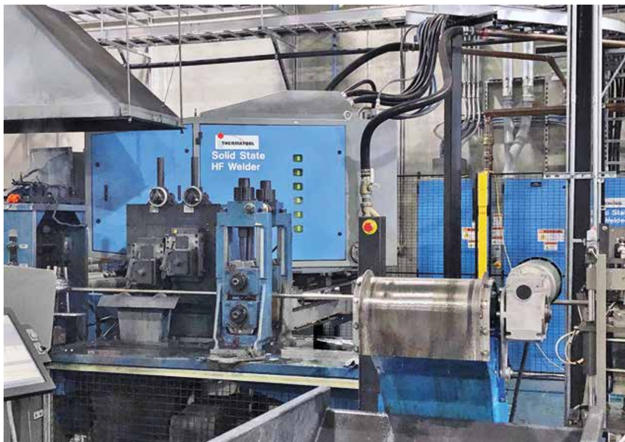
Thermatool CFI HF Welder
