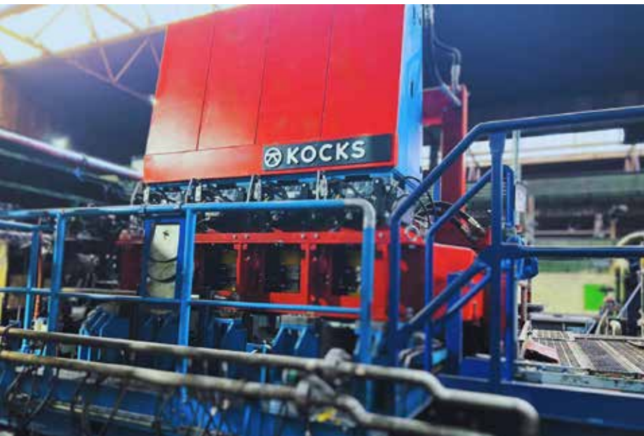
The KOCKS 4-roll stand with individually driven rolls
