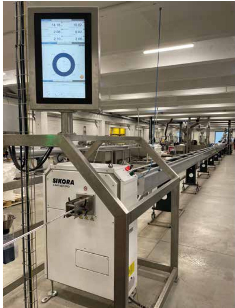
HÖHLE uses the X-RAY 6000 PRO for dimension measurement during the production of microducts
