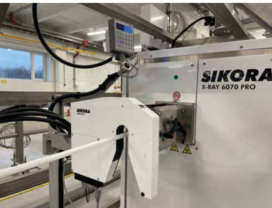
For utmost quality control HÖHLE includes the LUMP 2000 for lump and neckdown detection in the microduct extrusion lines
