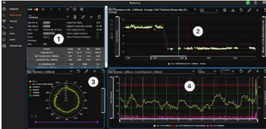
Figure 2 shows specific pipe identification and characteristics (zone 1); Historical data and batch trends (zone 2); pipe radial illustration (zone 3) and current tube longitudinal wall thickness and eccentricity profiles (zone 4).
