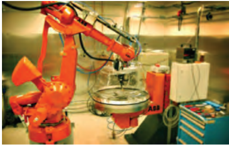
Figure 6. Small flexible system. The robot/ enclosure interface is effectively sealed against leaks using an adaptable occlusion. Enclosures up to 27 m 3 volume have been manufactured to accommodate large systems
