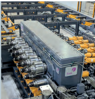
Fives Bronx Ltd – Bronx straightener for the ship building industry
