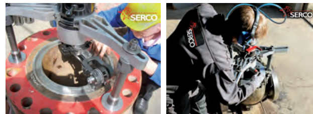
Portable lathe – flange & valve facing and boring machining units
