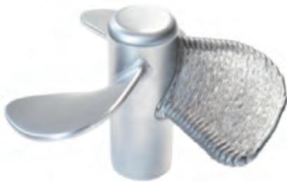
Figure 2. Propeller 200 x 240 x 240 mm. Material: 1.5125 G3Si1.
