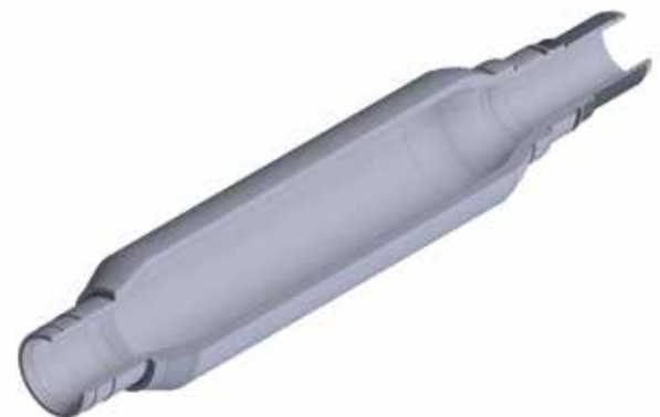
Preform, realized by cold rotary swaging
