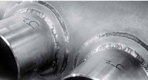
Zirconium alloy welded with effective inert gas protection showing no discolouration
