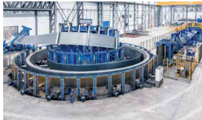
Horizontal Strip accumulator, 28-inch ERW tube welding line at Zekelman Industries, Blytheville, USA
