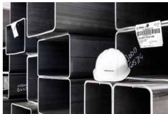
Square and rectangular hollow sections ranging from 8x8 inches to 22x22 inches produced on the 28-inch ERW tube welding line at Zekelman Industries, Blytheville, USA
