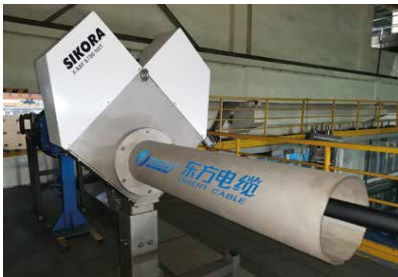
Ningbo Orient uses the X-RAY 8700 NXT from SIKORA in its submarine cable production line for final quality control
